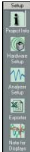
Fig. 2 The Setup task group with the measurement steps (from top) Project Information, Hardware Setup, Analyzer Setup and Exporter. There is also a note with information on displays
